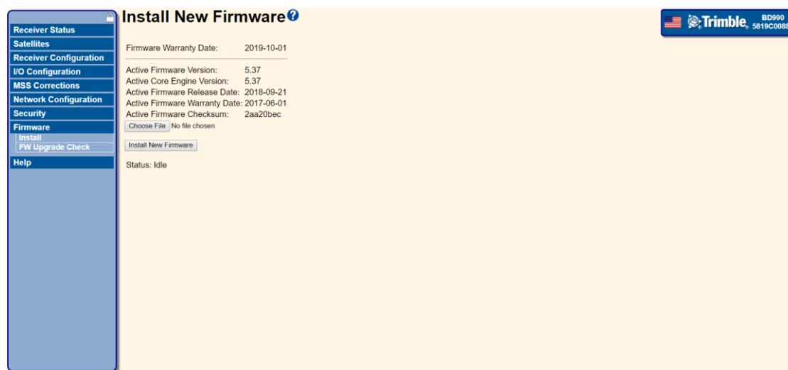
This page provides a summary of the firmware currently installed on the receiver. You can also use it to install new firmware on the receiver.
